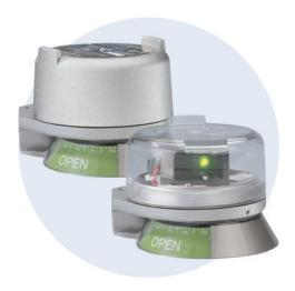
The YH, YO & YE Series offers one of the most versatile platforms for adapting to a variety of valve systems. The explosion/flame proof design is CSA/FM approved and ATEX certified for use in hazardous environments. With the epoxy coated anodized aluminum enclosure it may be used in corrosive heavy wash down areas as well.
