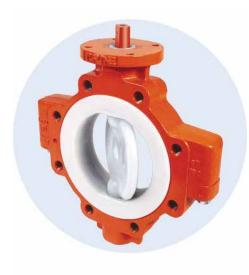
The XLD Series are PFA lined (up to 12") and PTFE lined (14" to 24") butterfly valves. The body is epoxy coated ductile iron (non-wetted). They are available with Wafer style or Lug style 150# ANSI flange connections. They can be equipped with a manual lever or can be actuated with electric or pneumatic actuators.
