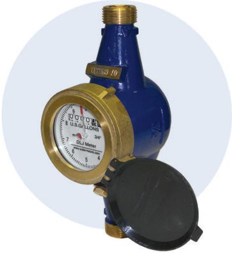
The WM Series water meters are multi-jet (inferential) impeller meters. They measure total flow in gallons. The impeller and magnet are the only moving parts in the measuring chamber. The chamber is located in a strainer basket, which allows for high amounts of impurities to be passed through the meter without affecting its operation. The impeller movement is transferred by a magnetic coupling to the hermetically sealed register.
