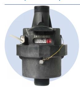
The WM-PD series water meters are volumetric piston displacement water meters. These meters use a mechanical transmission to advance a hermetically sealed, 8-digit register. They are suitable for use with potable cold water, and hot water. There are two sizes available, 1/2 inch and 3/4 inch.
