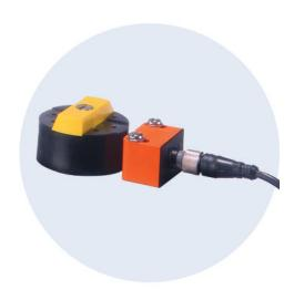
The UA/UB Series solid state proximity switch is a target puck with position indicator, two red LEDs and two solid state switches (N/O and 1 open, 1 closed).
