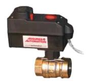
The on/off models operate by rotating 90° when power of the appropriate voltage is applied to the green control signal wire (see wiring diagram on label). When power is removed from the control signal, the actuator rotates back 90° to the original position. This is the "normal" or "signal de-energized" position, and can be changed in the field by rotating the square stem insert in the actuator's star shaped drive.
