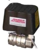
The modulating models operate by rotating from 0 to 90° in direct relation to the voltage applied to the green control signal wire.
