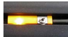
switch is closed and LED is lit
